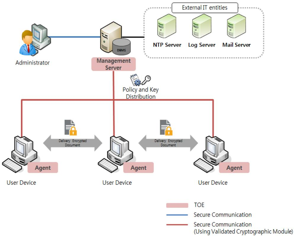
[Figure 1] Operational environment of Electronic Document Encryption (1)
