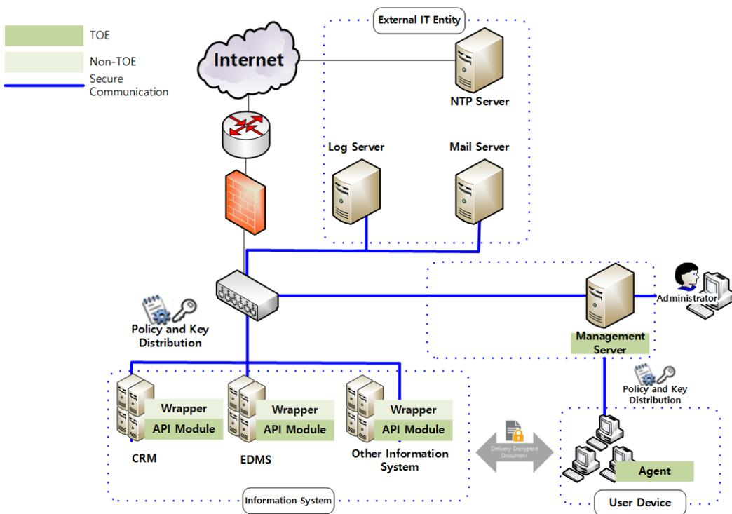
[Figure 2] Operational environment of Electronic Document Encryption (2)
