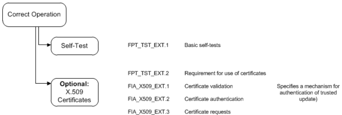
Figure 3: Correct Operation SFR Architecture
