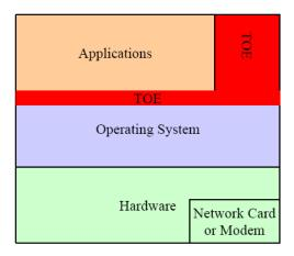
The TOE is used to regulate the flow of network traffic to and from the environment in which it is installed. As the TOE is connected to the Internet, the types of traffic that is regulated are:
