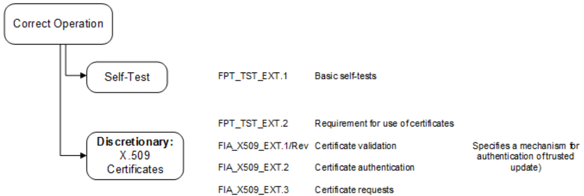
Figure 16: Correct Operation SFR Architecture
