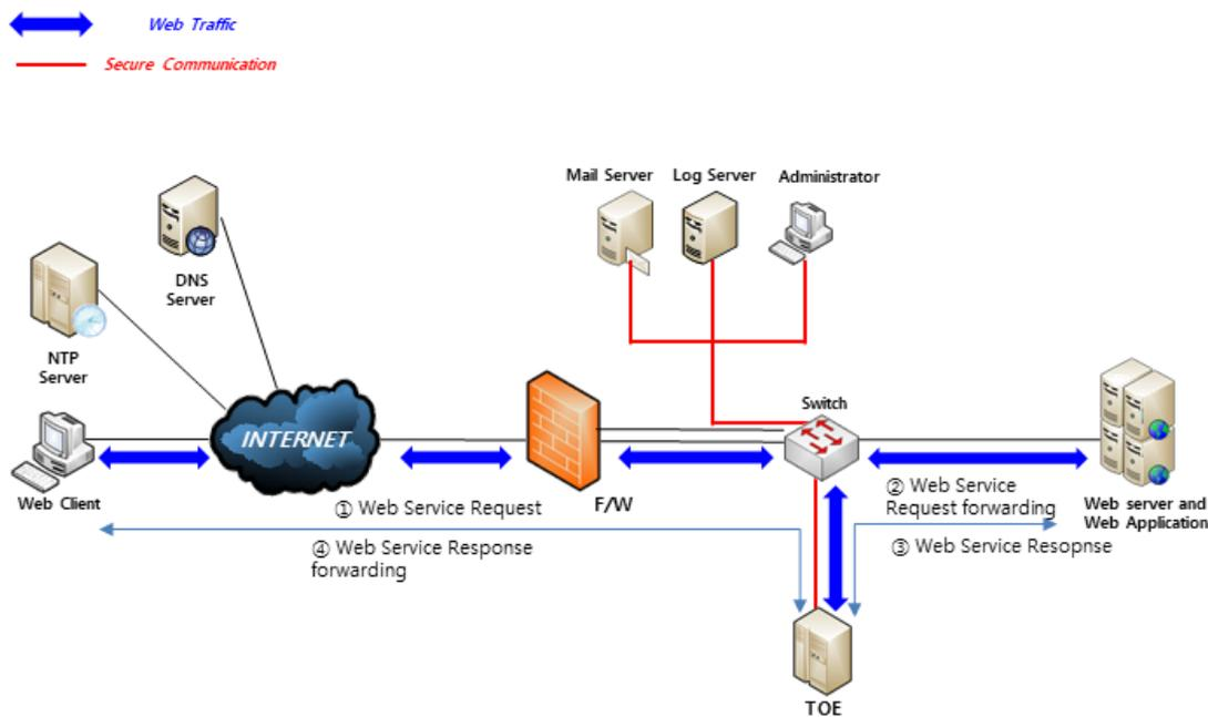
[Figure 2] Operational environment of the TOE (example: Reverse Proxy)
