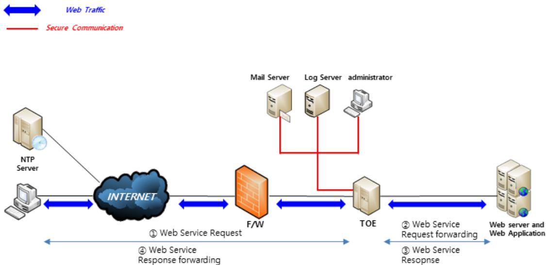
[Figure 1] Operational environment of the TOE (example: In Line)
