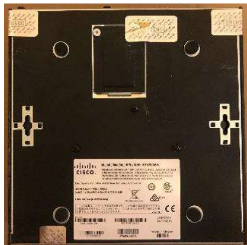
Figure 26 ASA 5506H-X Bottom TEL Placement
