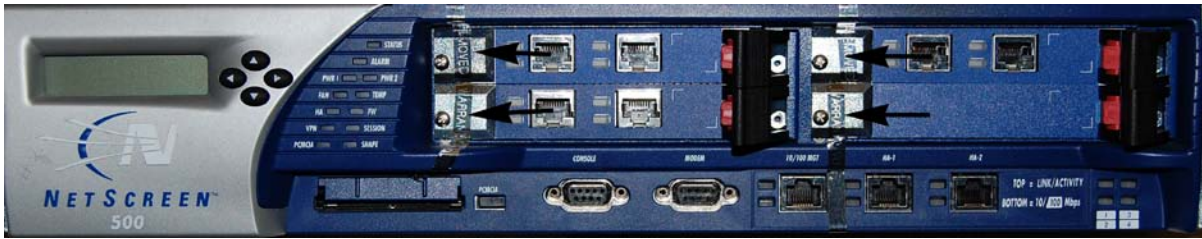
Figure 1: Front of the NetScreen-500, with location of tamper evident seals
