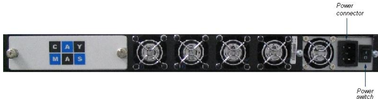
Figure 4 – 318 Rear Physical Ports
