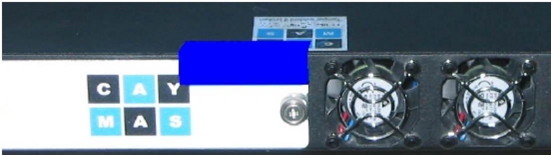
Figure 7 – Apply label to upper hard drive bay of the rear of the 318
