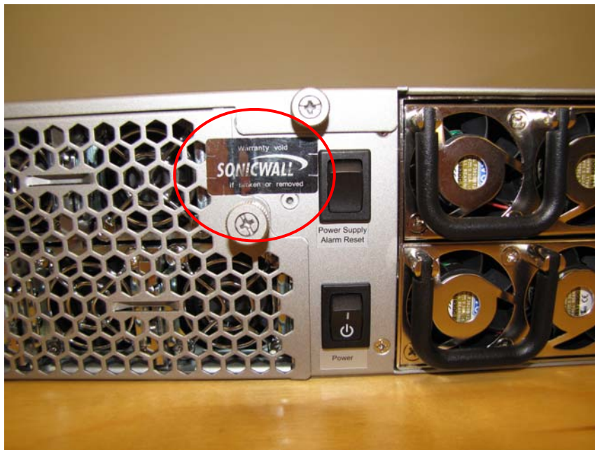
Figure 5 Tamper Seal #5 – Rear Fans
