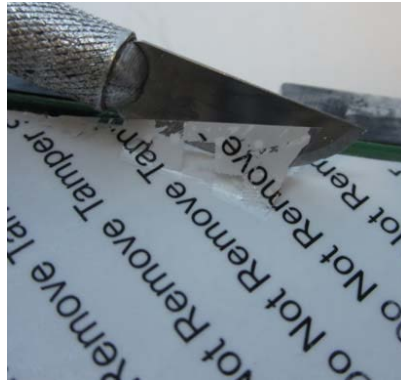
Figure 3: Tamper Evidence on Tamper Seal
