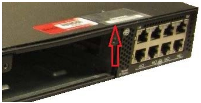
Figure 8 – Label #2 (Applied over Chassis Screw near Front/Right Corner)
