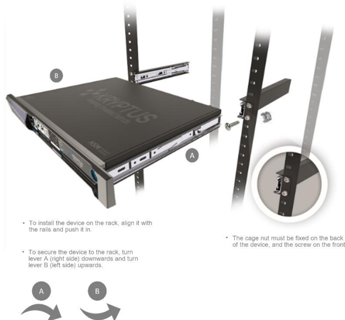
Figure 7: Installation on the rack
