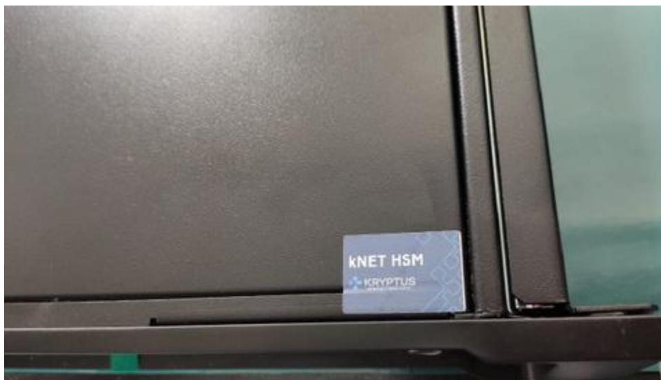
Figure 9: Tamper-evident seals – zoom in
