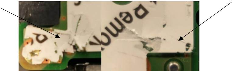
Figure 8 - Tamper Evidence on Tamper Seal
