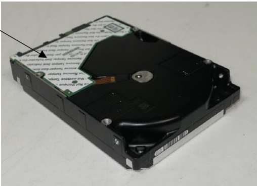
Figure 7 - Tamper-Evident Seal for Ultrastar DC HC555
