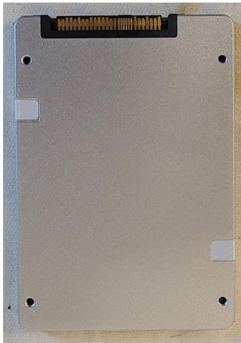
Figure 10 - Phison PASCARI-X100 series and Nytro-series U.2 7mm Module Seal Application Locations
