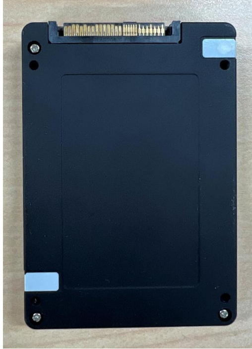
Figure 11 - Phison PASCARI-X200, X201, D205V and D206V series U.2 15mm Module Picture Seal Application Location
