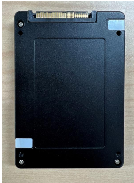
Figure 12 - Phison PASCARI-X200,D205V and D206V series U.2 15mm for larger capacities Module Seal Application Locations
