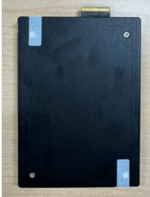
Figure 13. Phison PASCARI-X200, X201, D205V and D206V series E3.S Module Seal Application Locations
