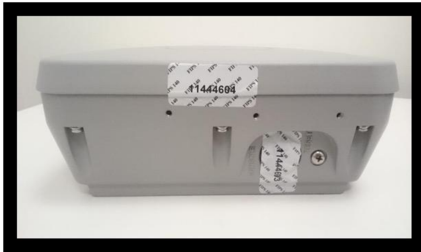
Figure 27: TEL Placement 4 and 5
