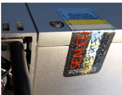
Figure 9: Tamper-Evident Seal X-Module Back
