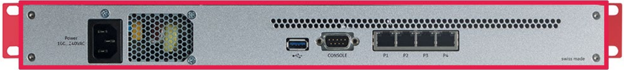
Figure 2: E-Module Back with Cryptographic Boundary in Red
