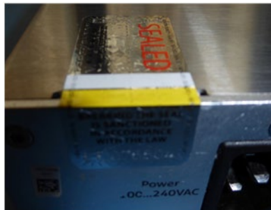
Figure 7: Tamper-Evident Seal (2) E-Module Back
