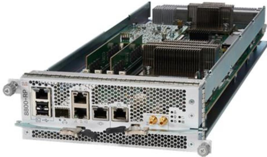
**Figure 3: Route Processor card (8800-RP)**
