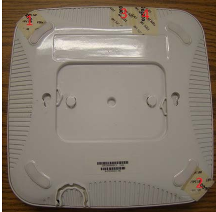
Figure 7 Required TELs for the Aruba 7005 Mobility Controller – Bottom
