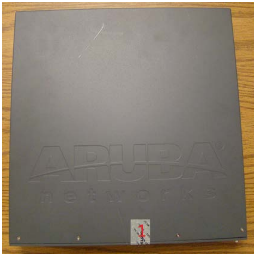
Figure 9 Required TELs for the Aruba 7010 Mobility Controller – Top
