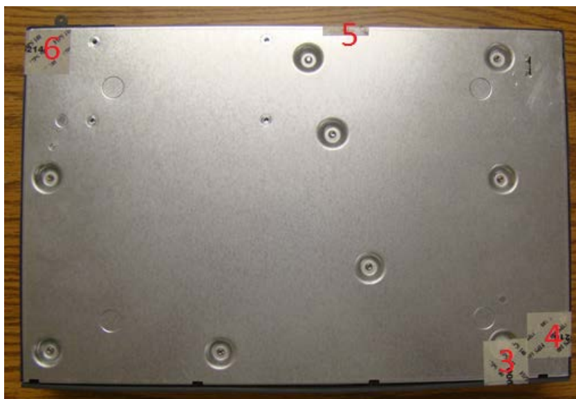
Figure 21 Required TELs for the Aruba 7205 Mobility Controller – Bottom
