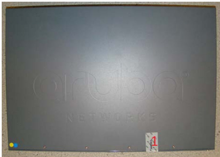
Figure 13 Required TELs for the Aruba 7024 Mobility Controller – Top
