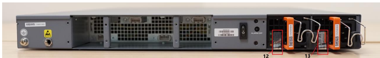
Figure 17 - SRX4100 & SRX4200 Rear View: TEL 12-13
