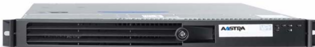
Figure 5: The ViPr Application Server (VAS)
