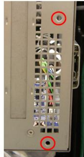
Figure 8 Small Louver Alignment
