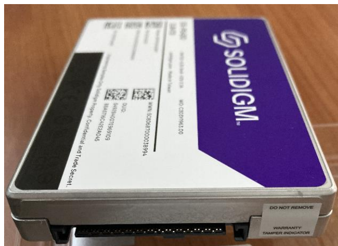
Figure 2 – U.2 Module Picture (Solidigm Branding)
