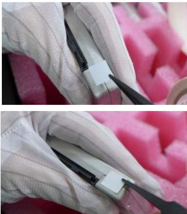
Figure 8 - Applying Tamper-Evident Seals
