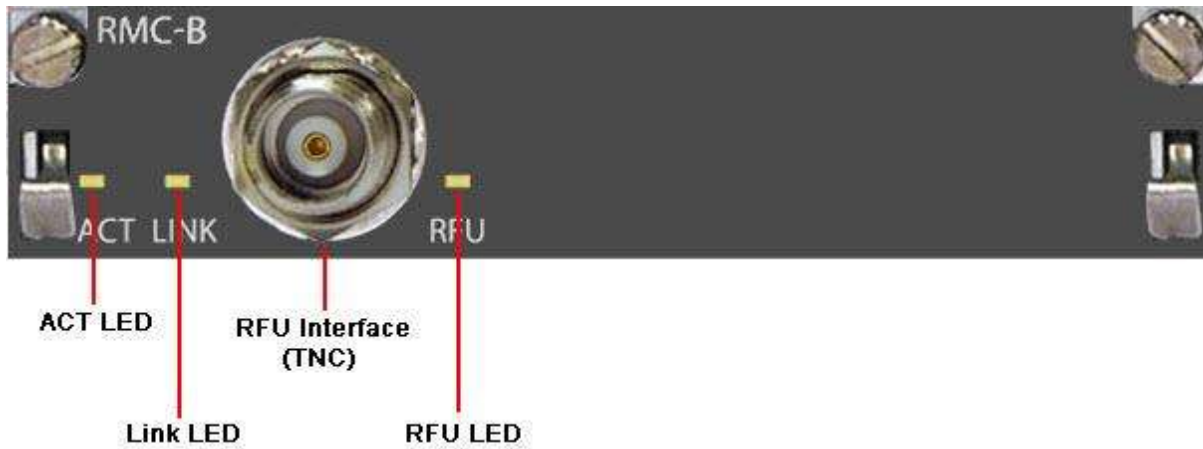
Figure 8 - PTP820 RMC-B: N000082H004 Interfaces
