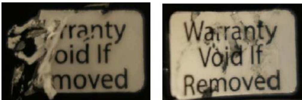
Figure 9 - Tamper Evidence on Tamper Seal
