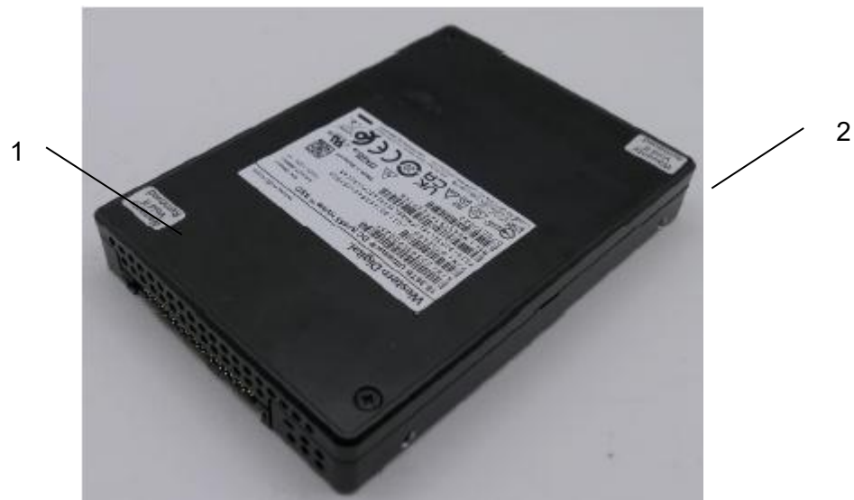
Figure 7 - Tamper-Evident Seals Ultrastar DC SN655, Top View
