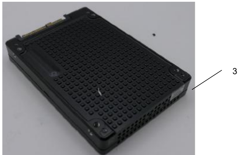
Figure 8 - Tamper-Evident Seal Ultrastar DC SN655, Bottom View and UART Access Point
