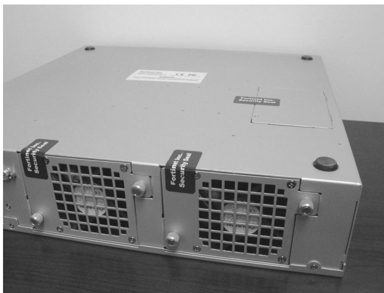
Figure 4: FortiGate-3000 and 3600 tamper seal placement
