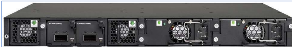
Figure 2 - Back side of ICX7450-48P with IPsec module inserted
