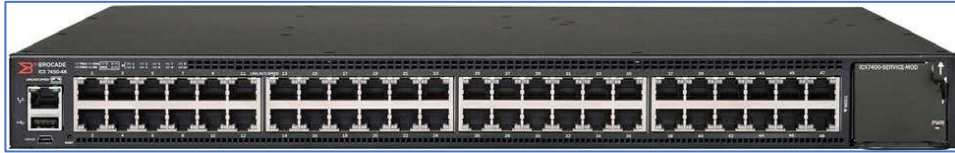
Figure 1 - Front/top side of ICX7450-48P with IPsec module inserted
