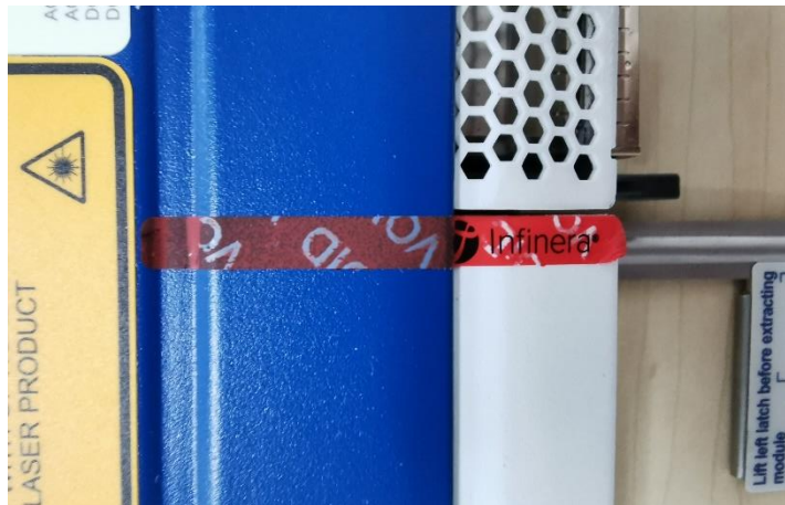
Figure 5 – Tamper-evident label: broken
