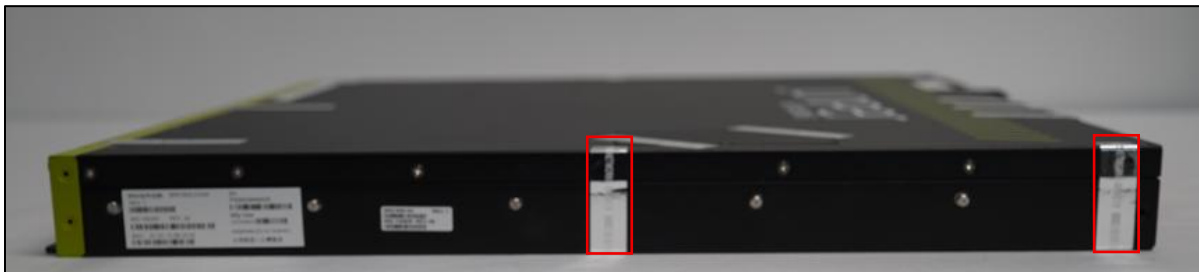
Figure 5 - SRX1600 Right Side View: TEL 4 and 5
