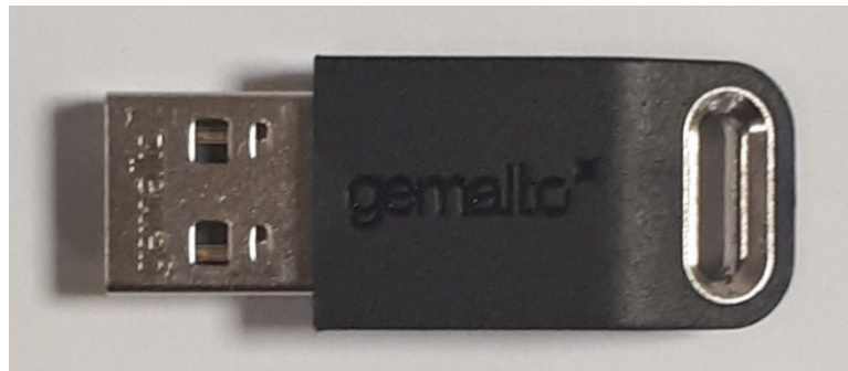
Figure 3 – eToken 5300 Mini with Outer Enclosure
