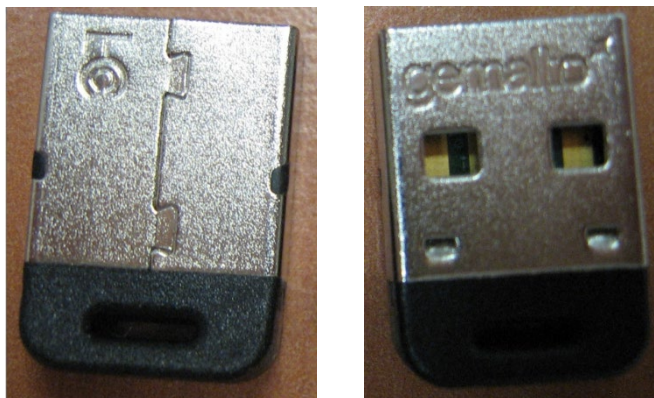
Figure 1 – 5300 Micro Crypto Boundary
