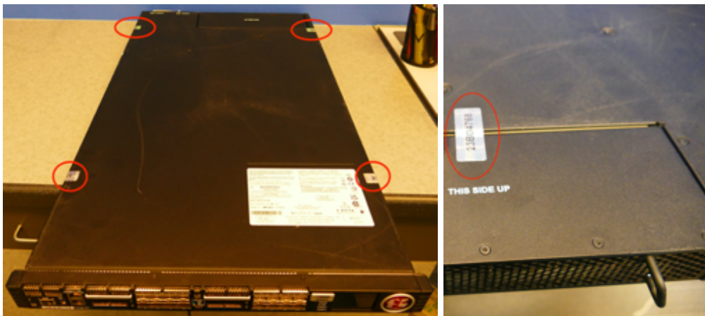
Figure 10 - Tamper labels on r10900, r10920-DF and r12900-DS (4 +1 of 5 tamper labels shown). Labels are located on the lateral sides of the platform -labels 1,2,3 and 4. The tamper label 5 on the chassis / enclosure lid is covering the ventilation fan tray that allows access to SSD.
