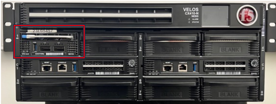
Figure 5 - VELOS CX410 BX110 with 7 filler panels and one blade. The BX110 tested blade in slot #1 delineated with red rectangle.
