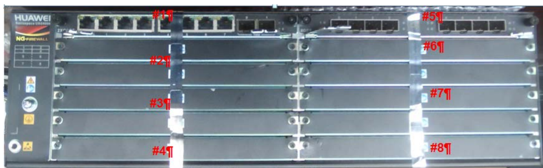
Figure 6-15 USG6650/USG6680 tamper seal placement- back
