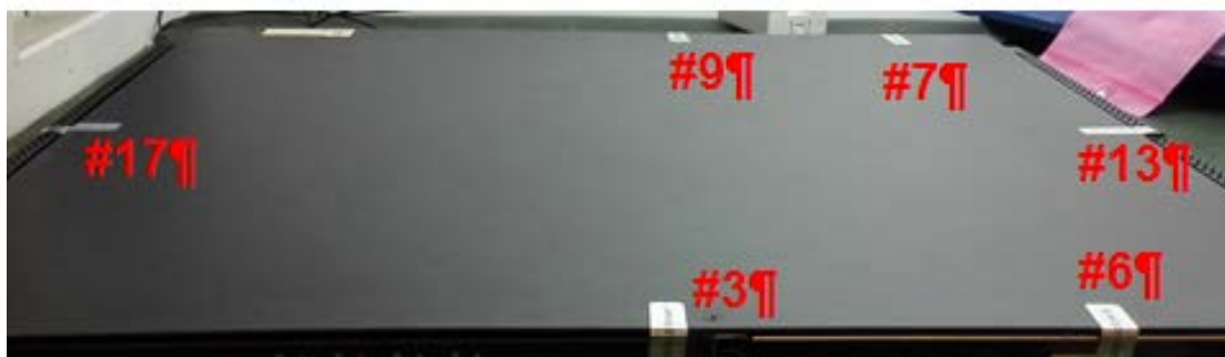
Figure 6-13 USG6370/6620 tamper seal placement- bottom
