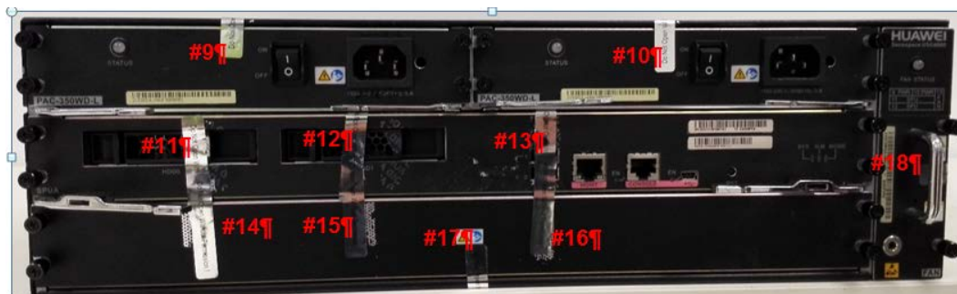
Figure 6-15 USG6650/USG6680 tamper seal placement- back
