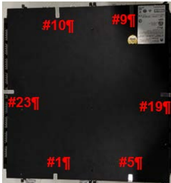
Figure 6-18 USG6650 /USG6680 tamper seal placement- top
