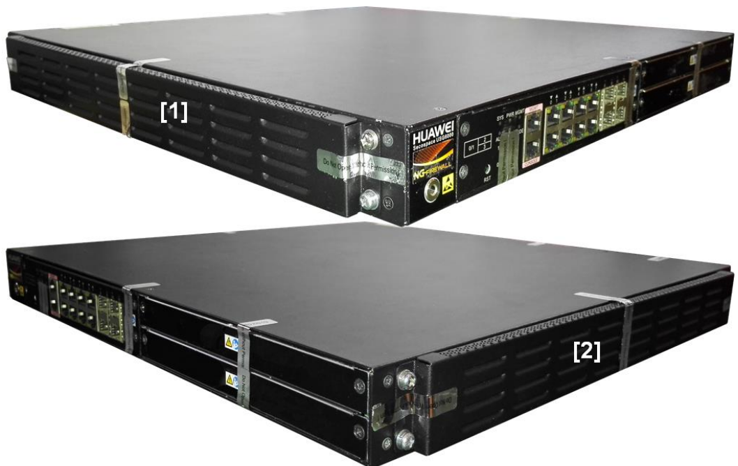
Figure 6-2 USG6370/6620 external baffle placement
