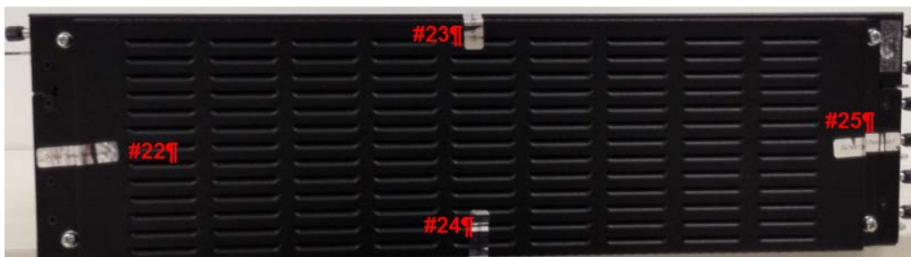
Figure 6-17 USG6650/USG6680 tamper seal placement- left side
