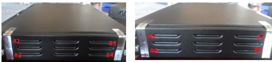
Figure 6-5 USG6310S tamper seal placement- right and left sides
