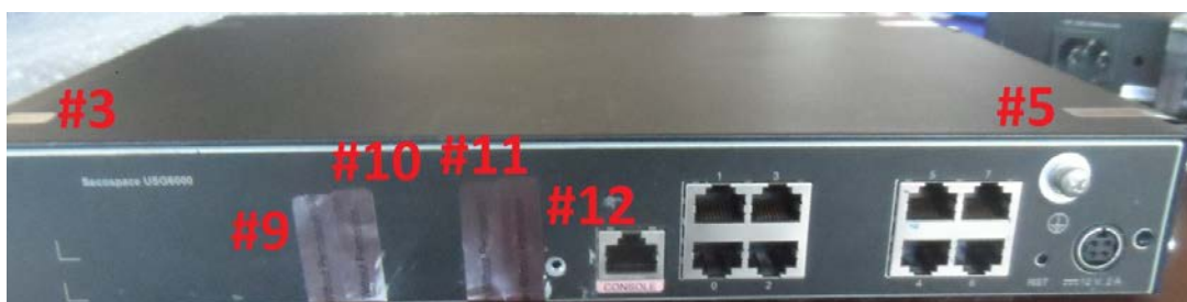
Figure 6-6 USG6310S tamper seal placement- back
