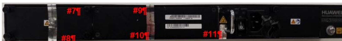
Figure 6-9 USG6370/6620 tamper seal placement- back
