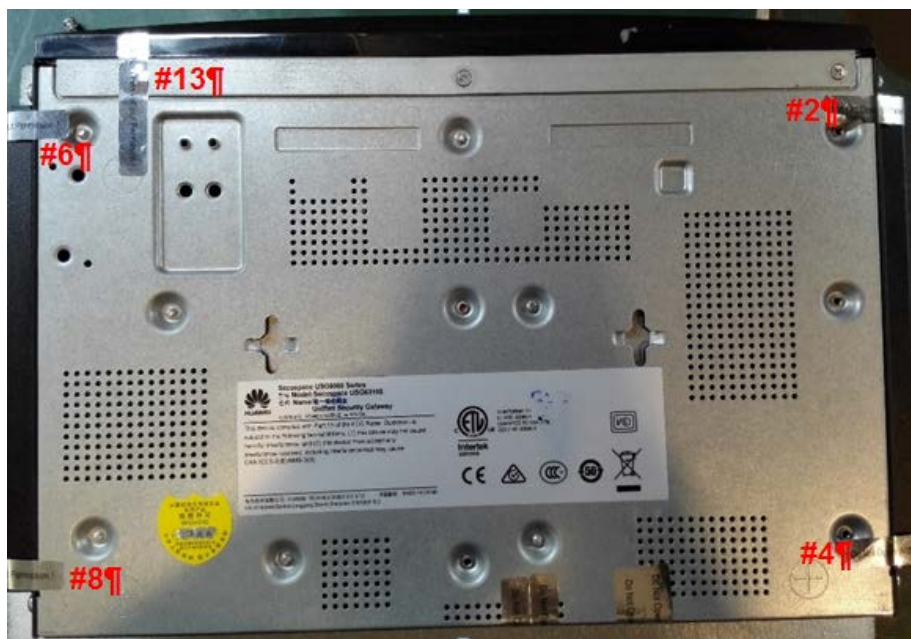
Figure 6-7 USG6310S tamper seal placement- bottom
