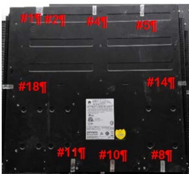
Figure 6-13 USG6370/6620 tamper seal placement- bottom
