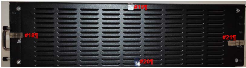
Figure 6-16 USG6650/USG6680 tamper seal placement- right side
