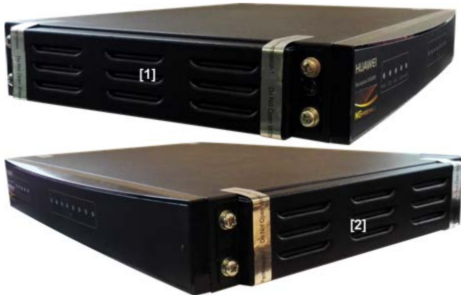
Figure 6-1 USG6310S external baffle placement
