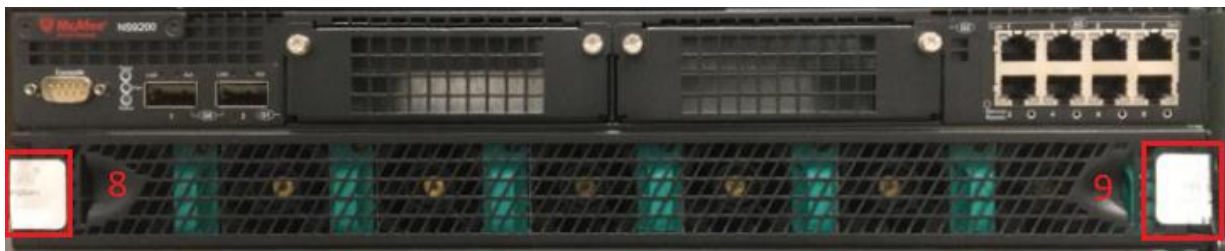
Figure 8 – Tamper Label Placement Front (NS9300 P sensor)
