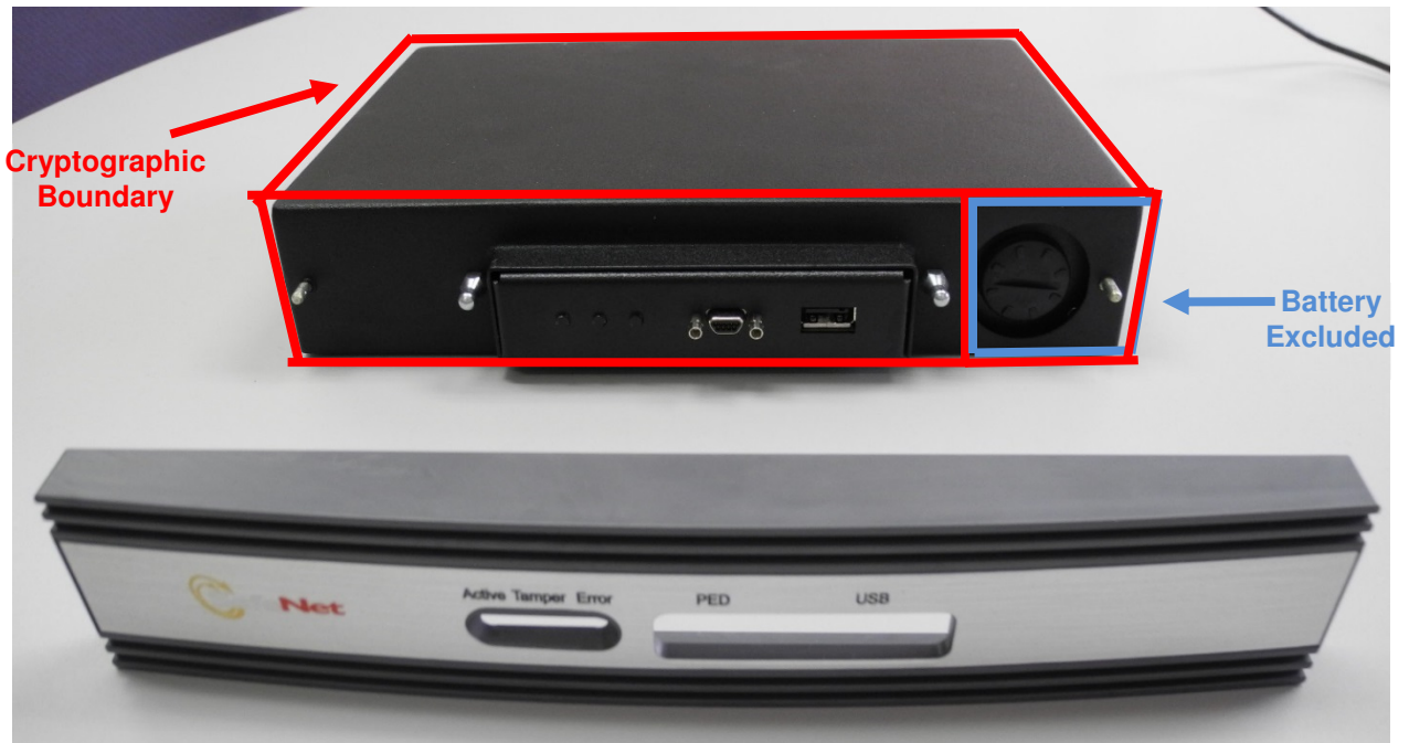
Figure 2-2. Thales Luna USB Cryptographic Boundary (with front bezel removed)
