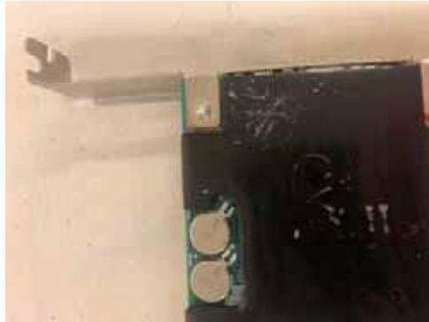
Figure 3 Cryptographic Module Showing Tamper Evidence
