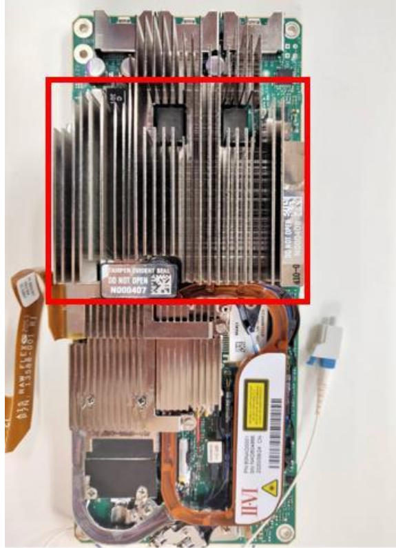
Figure 2: Cryptographic Boundary of WaveLogic 5 Extreme Encryption Modem (represents all P/Ns in Table 2)
