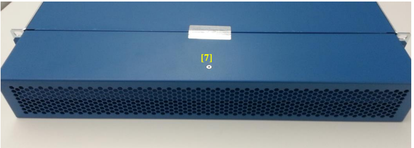
Figure 11 – PA-3060 Front/Top Tamper Seal Placement
