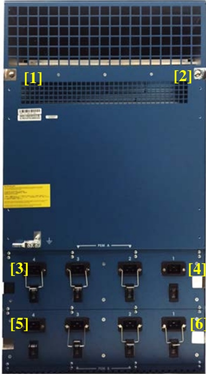
Figure 13 - PA-7080 Tamper Seal Placement for Rear (6)
