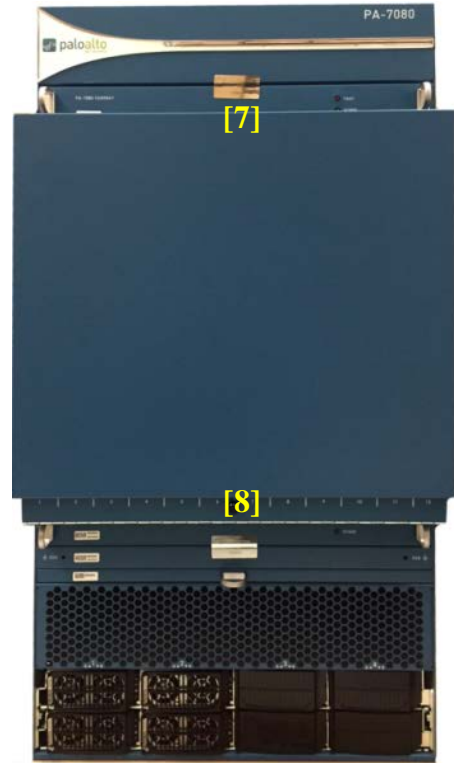
Figure 14 - PA-7080 Tamper Seal Placement on Front Fan Trays(2)
