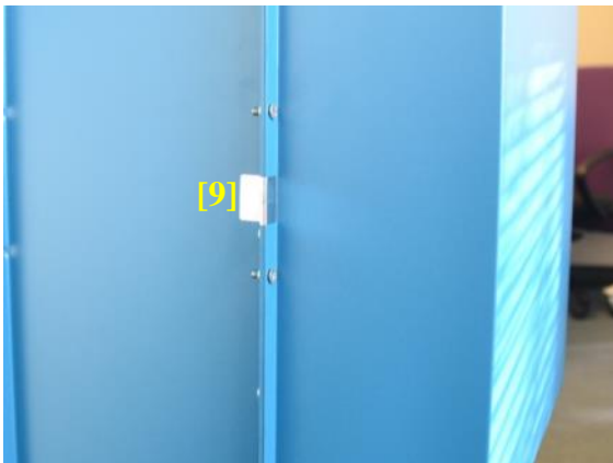
Figure 15 - PA-7080 Tamper Seal Placement on Left Side for Front Opacity Shield (1)
