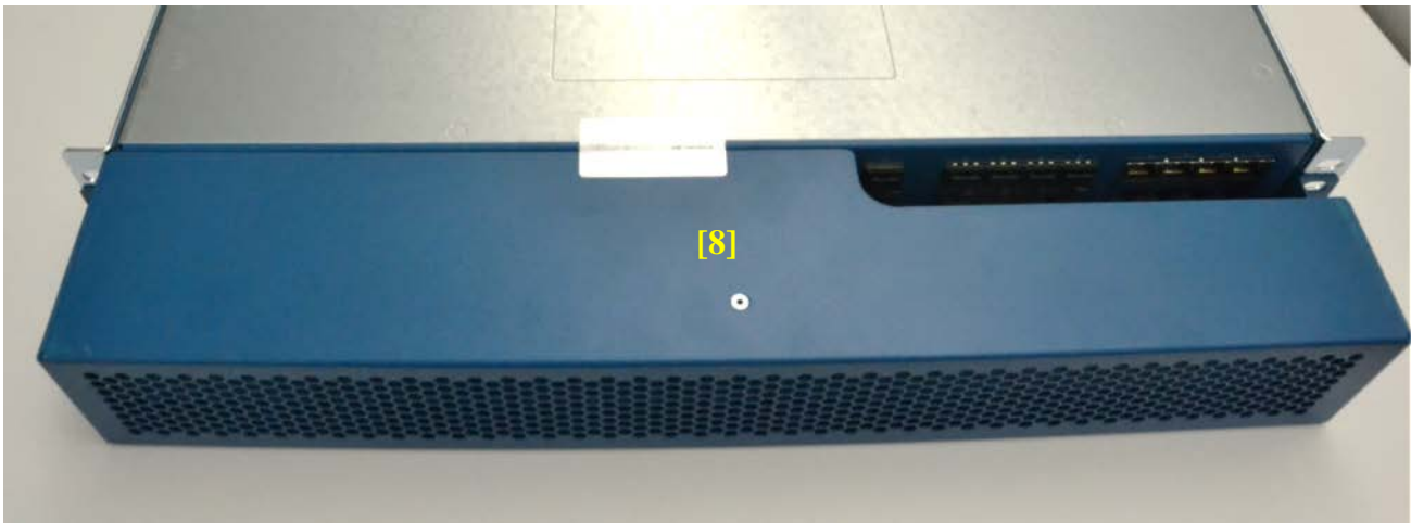
Figure 12 – PA-3060 Front/Bottom Tamper Seal Placement
