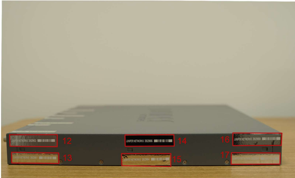
Figure 19 - SRX345 Dual-AC Tamper-Evident seal placement (RHS)
