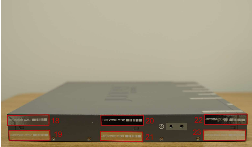
Figure 14 – SRX345 Tamper-Evident seal placement (RHS)
