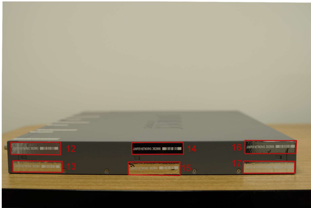
Figure 13 – SRX 345 Tamper-Evident seal placement (LHS)
