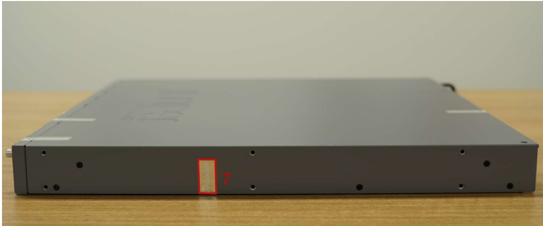
Figure 23 – SRX1500 Tamper-Evident seal placement (RHS)
