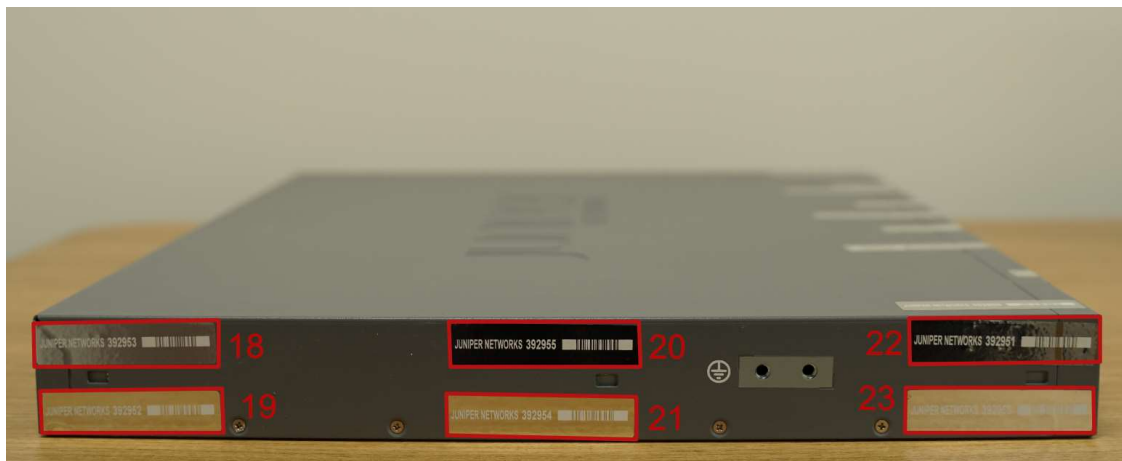
Figure 19 - SRX345 Dual-AC Tamper-Evident seal placement (RHS)
