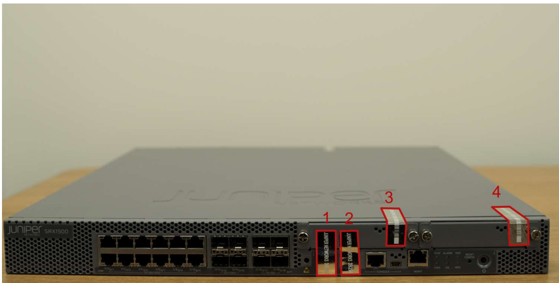
Figure 21 – SRX1500 Tamper-Evident seal placement (Rear)
