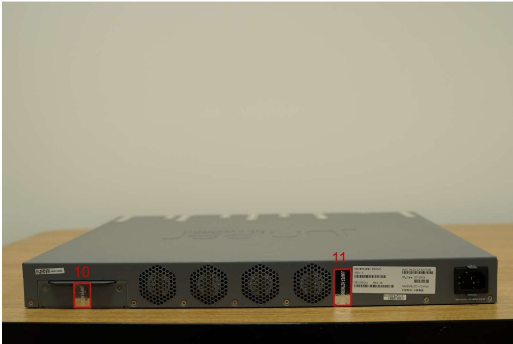
Figure 13 – SRX 345 Tamper-Evident seal placement (LHS)
