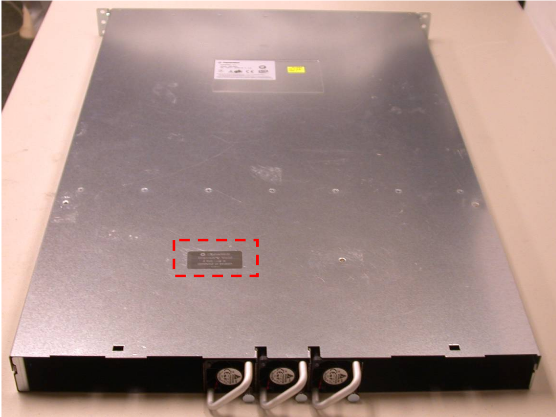
• Figure 2 – CM180D Tamper-Evident Seal Placement (shown in the red rectangle above)
