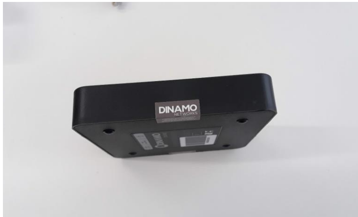
FIGURE 6 – EXAMPLE OF TAMPER-EVIDENT SEALS ADJOINING TOP AND BOTTOM OF POCKET ENCLOSURE
