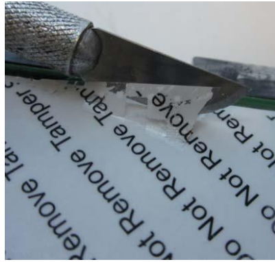
Figure 6: Tamper Evidence on Tamper Seal
