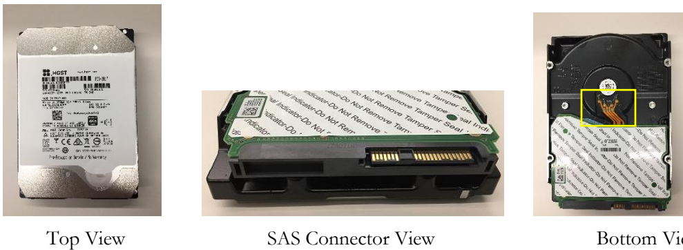
Figure 1: Ultrastar He 12 Cryptographic Boundary, Hardware Version 1
