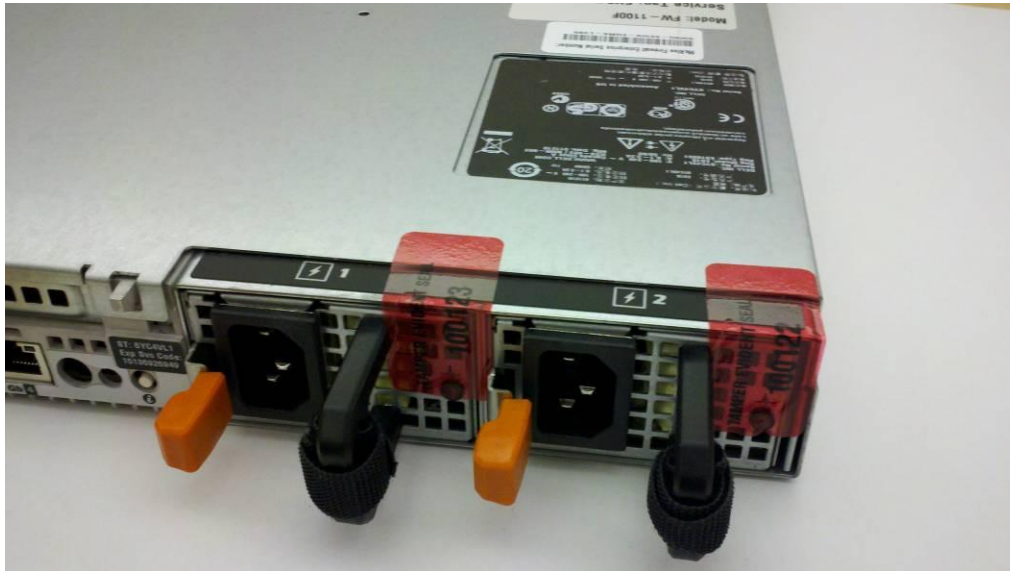
Figure 9 – Tamper-Evident Seal Application Positions (Power Supplies)
