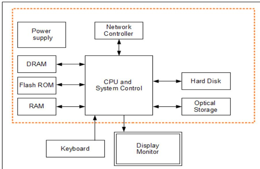
Figure 2: Oracle Linux UEK Hardware Block Diagram
