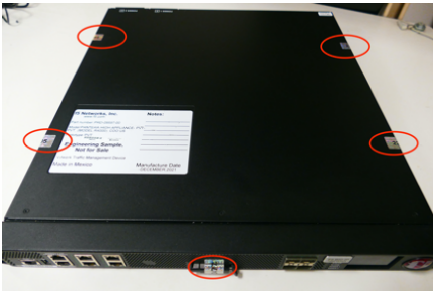
Figure 6 - Tamper labels on r4800 (5 of 5 tamper labels)
