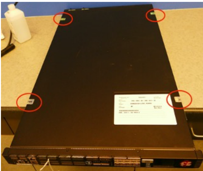
Figure 7 - Tamper labels on r5900 (4 of 4 tamper labels)
