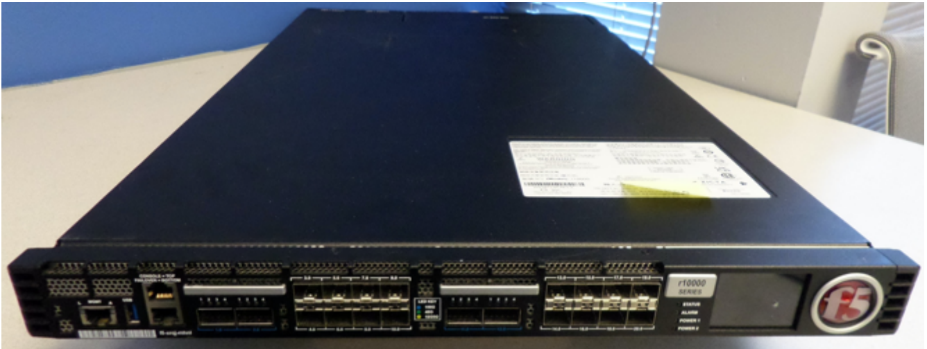
Figure 4 - r10900, r10920-DF front view (same chassis for the test platforms)
