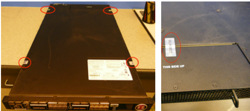
Figure 9 - Tamper labels on r10900, r10920-DF (4 +1 tamper labels shown). Labels are located on the lateral sides of the platform -labels 1,2,3 and 4. The tamper label 5 on the chassis lid is covering the ventilation fan tray that allows access to SSD.
