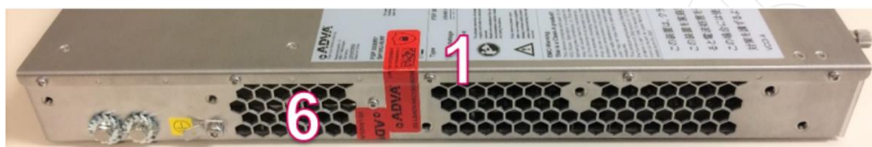
Figure 24: Placement of seals SH1HU-R/PF left side positions
