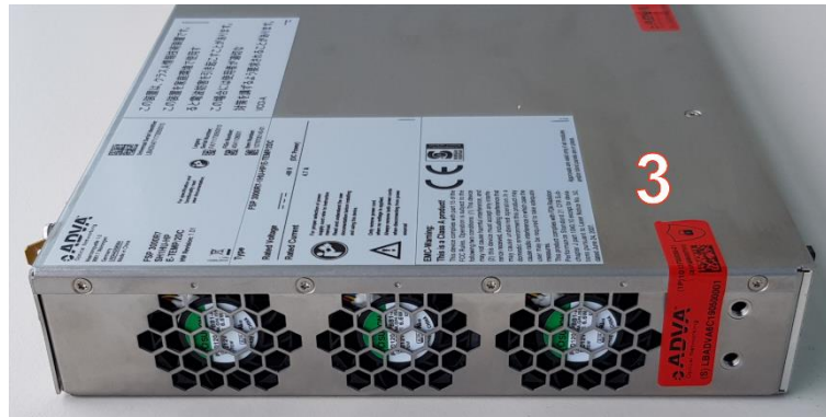
Figure 20: Placement seals, shelf 1 HU, placement 3
