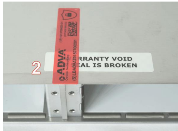
Figure 26: Placement of seal SH1HU-R/PF right side position
