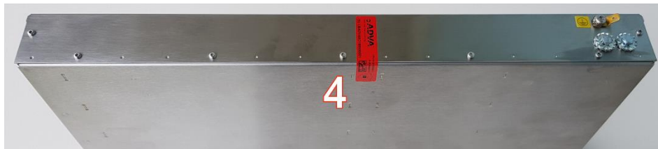
Figure 21: Placement seals, shelf 1 HU, placement 4
