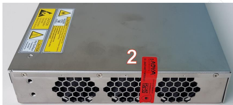
Figure 19: Placement seals, shelf 1 HU, placement 2
