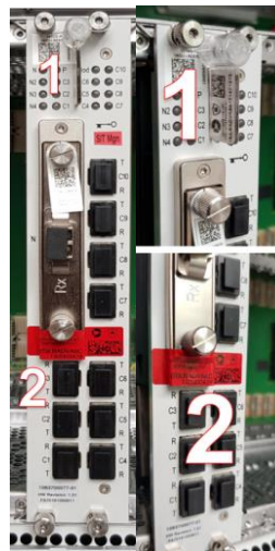
Figure 29: Placement of seals in SH9HU configuration
