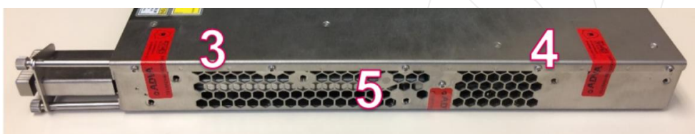
Figure 25: Placement of seals SH1HU-R/PF right side positions
