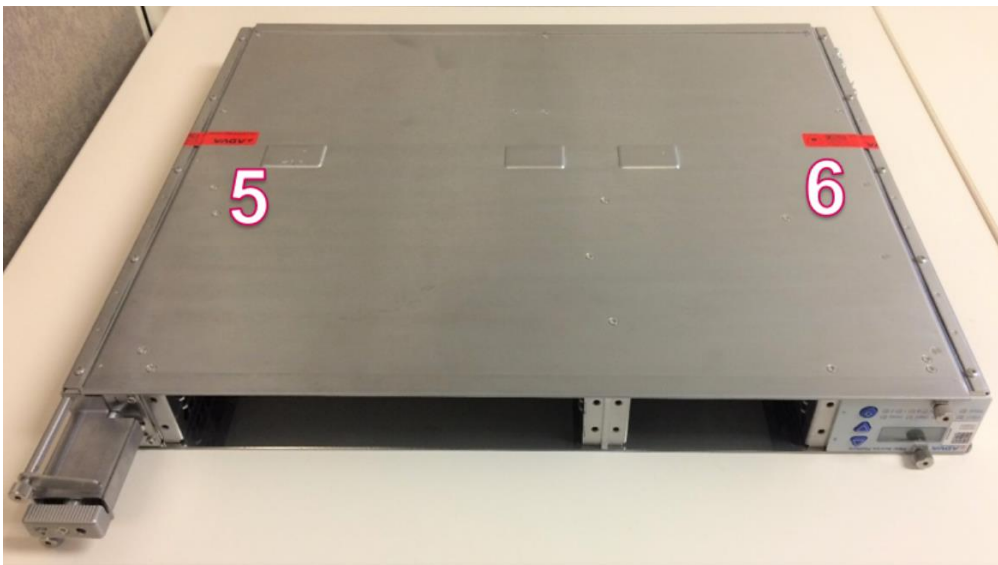
Figure 23: Placement of seals SH1HU-R/PF front-bottom
