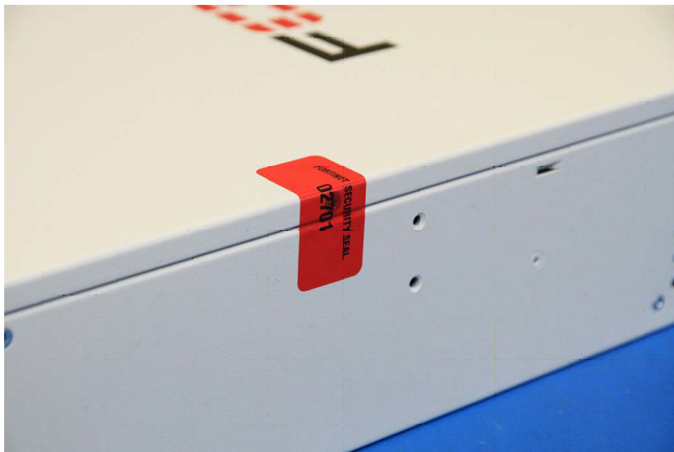
Figure 6: FortiManager-1000D external enclosure seal, top, left
