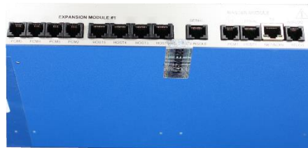
Figure 16: PA111-RM, PA155-RM, PA199-RM Tamper Seals at Rear/Bottom
