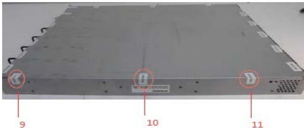
Figure 26 VDX 6740T-24, VDX 6740T-48 and VDX 6740T-64 bottom right side seal locations
