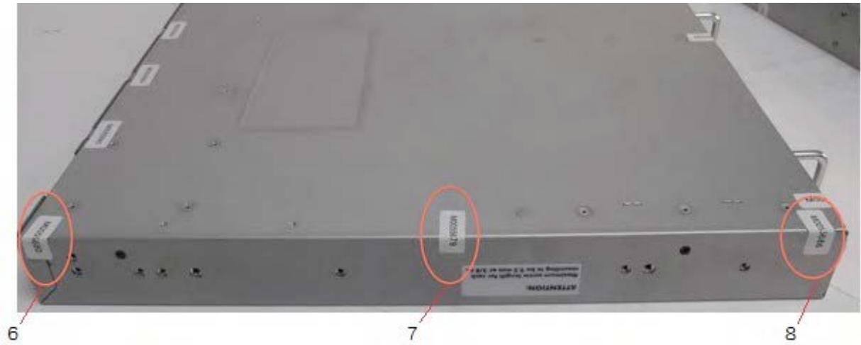
Figure 20 VDX 6740-24, VDX 6740-48 and VDX 6740-64-ALLSW bottom left side seal locations
