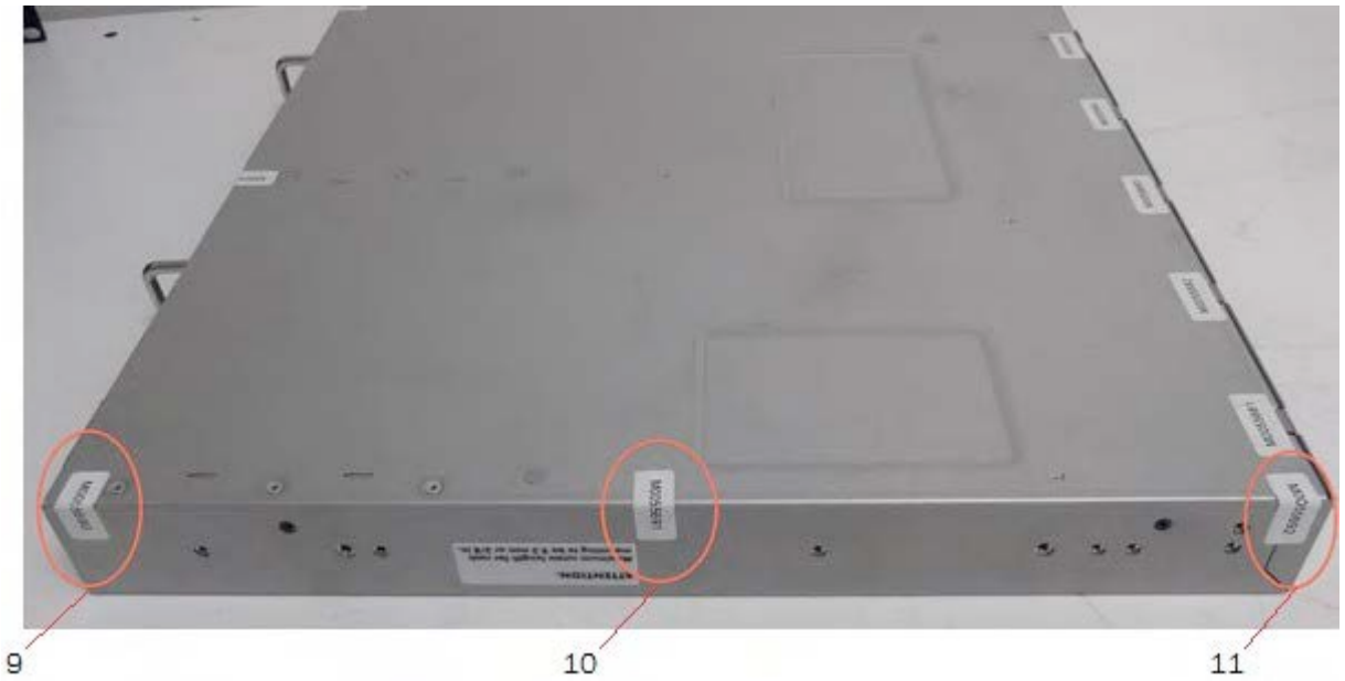
Figure 21 VDX 6740-24, VDX 6740-48 and VDX 6740-64-ALLSW bottom right side seal locations
