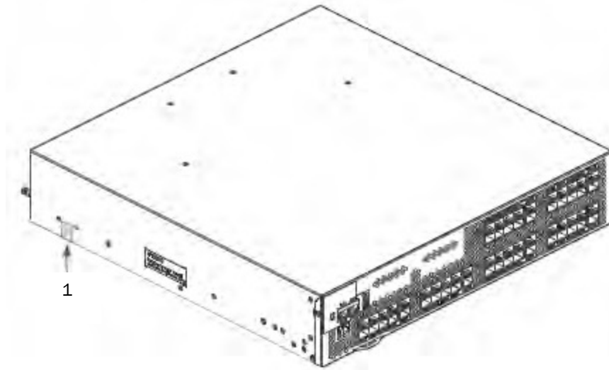
Figure 13 VDX 6720-40 and VDX 6720-60 left side seal location
