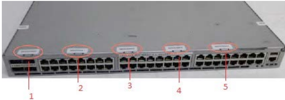
Figure 24 VDX 6740T-24, VDX 6740T-48 and VDX 6740T-64 bottom/front seal locations
