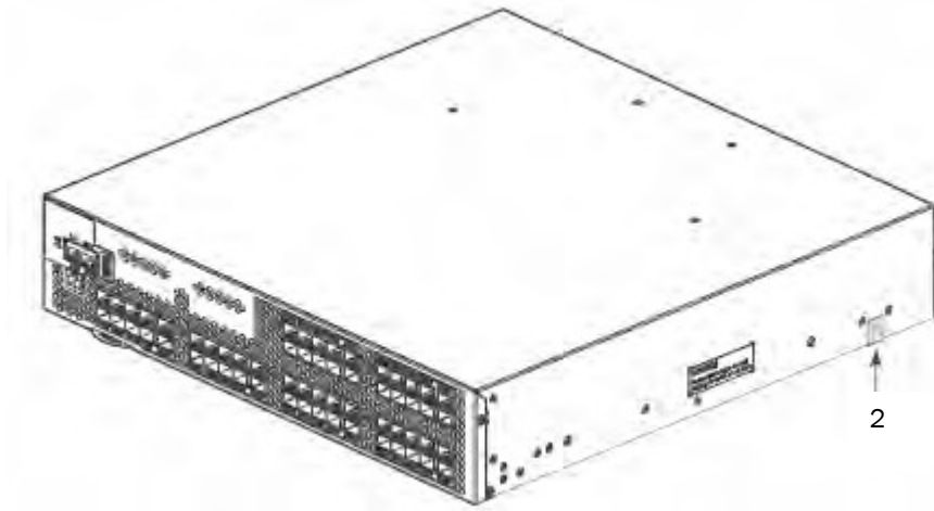
Figure 14 VDX 6720-40 and VDX 6720-60 right side seal location
