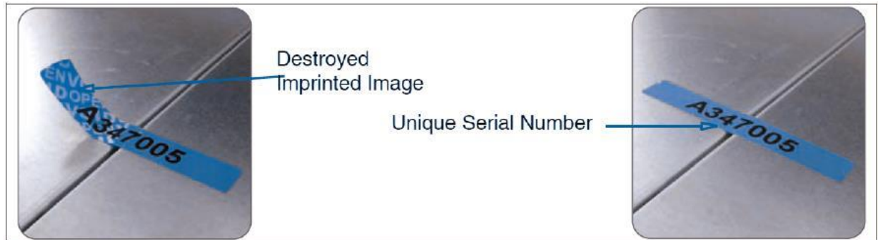
Figure 12 ASG S400 Labels Showing Tamper Evidence
