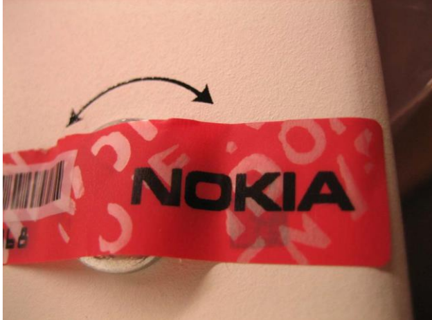
Figure 24 - Tamper-evident label: broken
