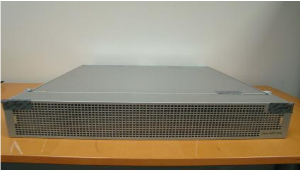
Figure 10: ASR 1002f with Opacity Shield Installed
